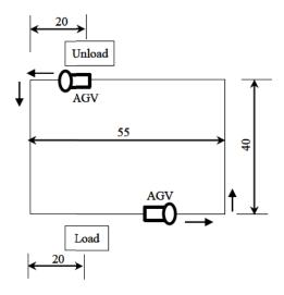
Considering a vehicle velocity of 50 m/min, availability of 0.95 and traffic factor of 0.9, the number of vehicles required to satisfy a demand of 50 delivery/hour is \_\_\_\_\_
