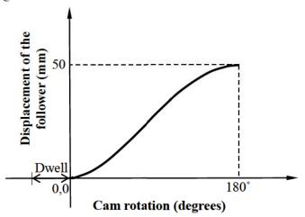
If the cam rotates at a uniform angular speed of 100 rpm, the speed of the follower (in mm/s) at the instance when the cam rotates  $45^{\circ}$  from the initial position is
