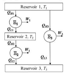
The efficiency of the engine  $\mathbb{E}_3$  in terms of the efficiencies  $\eta_1$  and  $\eta_2$  of the engines  $\mathbb{E}_1$  and  $\mathbb{E}_2$ , respectively, is
