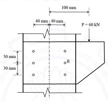
The resultant force in bolt R (in kN, round off to one decimal place) is \_\_\_\_\_
