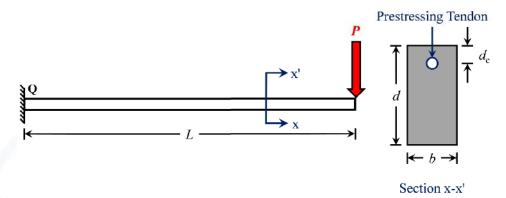
If the concentrated load, P = 5 kN, the resultant stress (in MPa, in integer) experienced at point 'Q' will be \_\_\_\_\_
