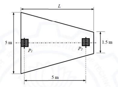
If the stress beneath the footing is uniform, the length of the combined footing L (in m, round off to two decimal places) is \_\_\_\_\_\_
