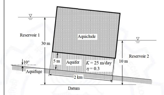
If water in Reservoir 1 is contaminated then the time (in days, round off to one decimal place) taken by the contaminated water to reach to Reservoir 2 will be
