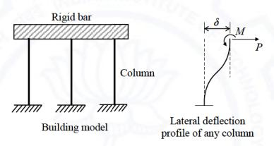
For the lateral deflection profile of the columns as shown in the figure, the natural frequency of the system for horizontal oscillation is
