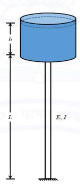
If elastic modulus (E) of steel is 200 GPa, ignoring self-weight of the tank, for the supporting steel column to remain unbuckled, the maximum depth (h) of the water permissible (in m, round off to one decimal place)
