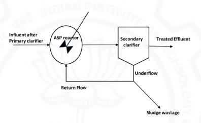
The underflow volume (in m³/day, round off to one decimal place) of sludge wastage is \_\_\_\_\_
