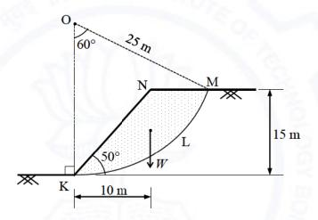
Considering the trial slip circle KLM, the factor of safety against the failure of slope under undrained condition (round off to two decimal places) is \_\_\_\_\_
