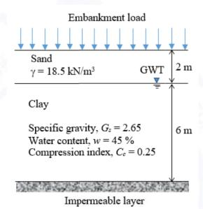
The primary consolidation settlement (in m, round off to two decimal places) of the clay layer resulting from this loading will be \_\_\_\_\_
