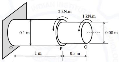
The absolute maximum shear stress in the member (in MPa, round off to one decimal place) is \_\_\_\_\_
