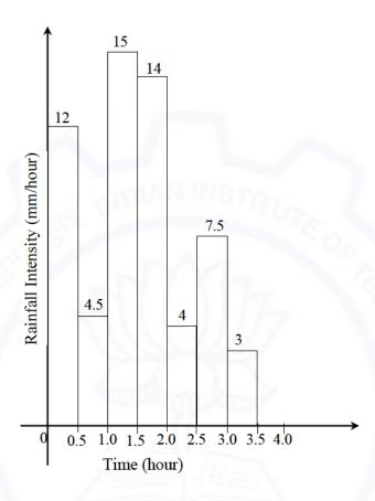
If the rainfall event has produced a direct runoff of 1.6 cm, the  $\phi$ -index of the event (in mm/hour, round off to one decimal place) would be
