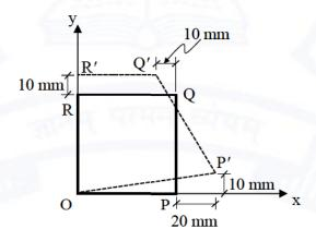
The horizontal displacement of the point (0.5 m, 0.5 m) in the plate O-P-Q-R (in mm, round off to one decimal place) is
