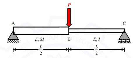
The mid-span deflection of the beam (in mm, round off to integer) under P = 100 kN in downward direction will be \_\_\_\_\_
