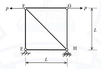
If  $R = 500 \times 10^3$  kN, P = 150 kN and L = 3 m, the magnitude of the horizontal displacement of joint G (in mm, round off to one decimal place) is
