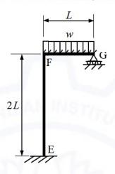
Considering the joint F being rigid, the support reaction at G is
