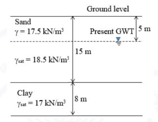
The overconsolidation ratio (OCR) (round off to two decimal places) at the mid-point of the clay layer is \_\_\_\_\_
