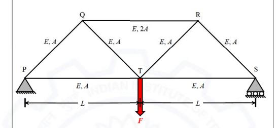
If load,  $F=10\sqrt{3}$  kN, moment of inertia,  $I=8.33\times10^6$  mm<sup>4</sup>, area of cross-section,  $A=10^4$  mm<sup>2</sup>, and length, L=2 m for all the members of the truss, the compressive stress (in kN/m<sup>2</sup>, *in integer*) carried by the member Q-R is
