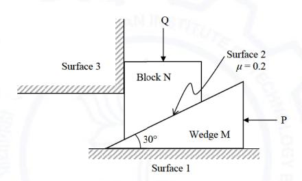
The limiting force P, in terms of Q, required for impending motion of block N to just move it in the upward direction is given as  $P = \alpha Q$ . The value of the coefficient ' $\alpha$ ' (round off to one decimal place) is
