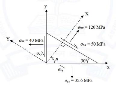
The absolute magnitude of the shear stress component  $\sigma_{xy}$  (in MPa, round off to one decimal place) in x-y coordinate system is
