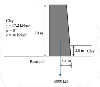
The factor of safety (round off to two decimal places) against sliding failure of the retaining wall after ignoring the passive earth pressure will be \_\_\_\_\_
