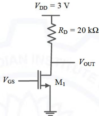
The channel length modulation coefficient is ignored. If the gate-to-source voltage  $V_{GS}$  is 1 V to keep the transistor at the edge of saturation, then the threshold voltage of the transistor (rounded off to one decimal place) is \_\_\_\_\_ V.
