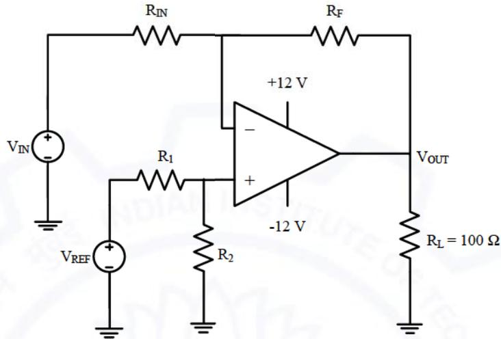
If  $V_{OUT} = 1$  volt for  $V_{IN} = 0.1$  volt and  $V_{OUT} = 6$  volt for  $V_{IN} = 1$  volt, where  $V_{OUT}$  is measured across  $R_L$  connected at the output of this OPAMP, the value of  $R_F/R_{IN}$  is
