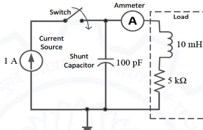
Initially, when the switch is open, the capacitor is discharged and the ammeter reads zero ampere. After the switch is closed, the ammeter reading keeps fluctuating for some time till it settles to a final steady value. The maximum ammeter reading that one will observe after the switch is closed (rounded off to two decimal places) is \_\_\_\_\_ A.
