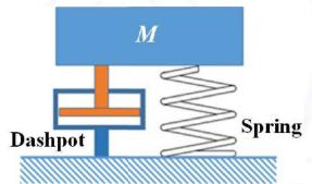
If the amplitude of the free vibration response reduces from 8 mm to 1.5 mm in 3 cycles, the damping ratio of the system is \_\_\_\_\_\_ (round off to three decimal places).
