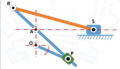
The quick return ratio for the mechanism is \_\_\_\_\_ (round off to one decimal place).
