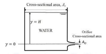
Neglecting any losses, the time taken by water in the tank to reach a level of y = H/4 is \_\_\_\_\_\_ seconds (round off to one decimal place).
