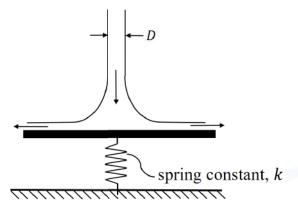
If the spring shows a steady deflection of 1 cm upon impingement of jet, then the velocity of the incoming jet is \_\_\_\_\_ m/s (round off to one decimal place).
