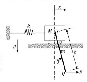
Assume that the spring deflects only horizontally and force F is applied horizontally at Q. For this system, the Lagrangian, L is
