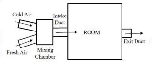
mass flow rate of the fresh air is 1.6 times of the cold air stream. Air leaves
