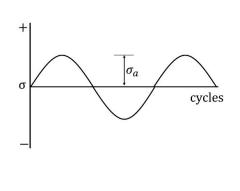
A specimen of this alloy is subjected to multiple stress cycles sequentially in the following order: (i) first 5000 cycles at  $\sigma_a = 400$  MPa followed by (ii) 25000 cycles at  $\sigma_a = 300$  MPa and finally (iii) at  $\sigma_a = 500$  MPa. Assuming that Miner's law is obeyed, the number of cycles to failure at the final applied stress of 500 MPa is \_\_\_\_\_\_.
